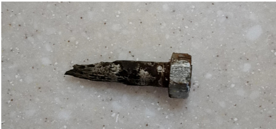
Photo: Pintle bolt after 40 years
