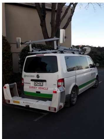
Figure 4 – 2: High speed data collection vehicle
