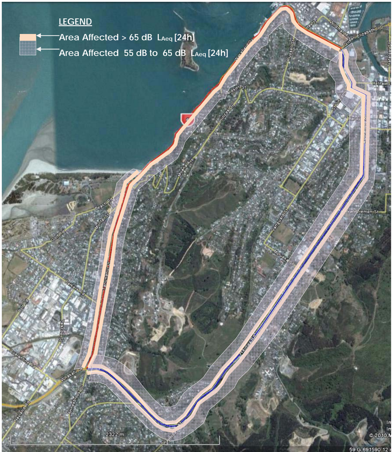
Figure 1 Predicted L_{Aeq} [24h] traffic noise levels based on the above 24 hour traffic volumes and average vehicle as per 'Do Minimum' 2036. Not to Scale
