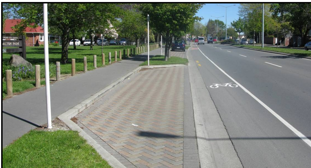
Figure 4-S Different Surfacing Provides Visual Separation between Parking Spaces and the Carriageway
